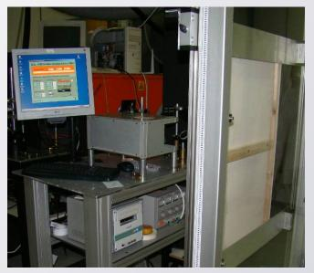
Laser cleaning workstation for the removal of polymeric coatings and/or over-layers from painted surfaces;
